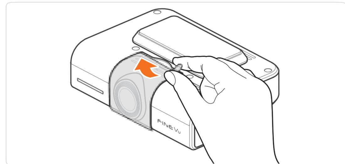
2. Remove the protective film from the front camera.
