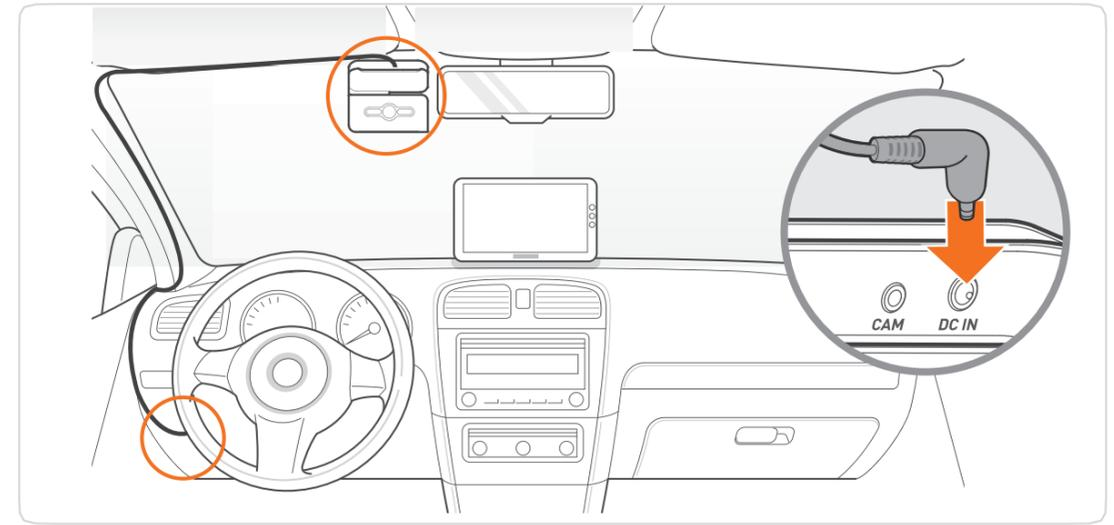
5. Connect to the constant power cable connected to the fuse box.
