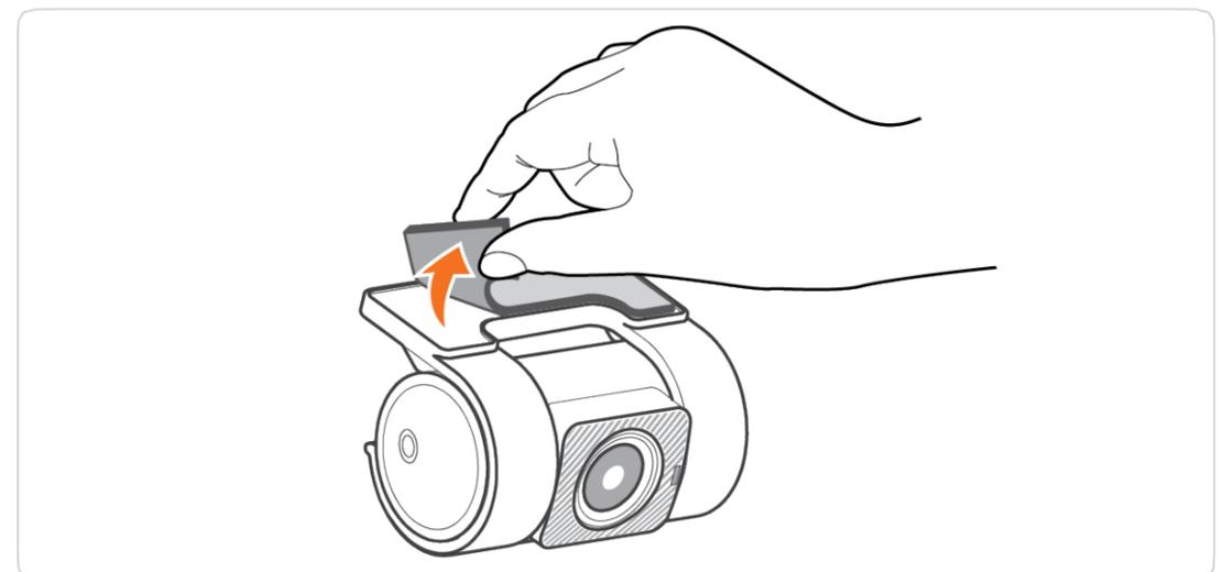
3. Peel off the protective film from the tape to attach the cradle.
