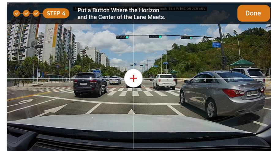
4. Align the
