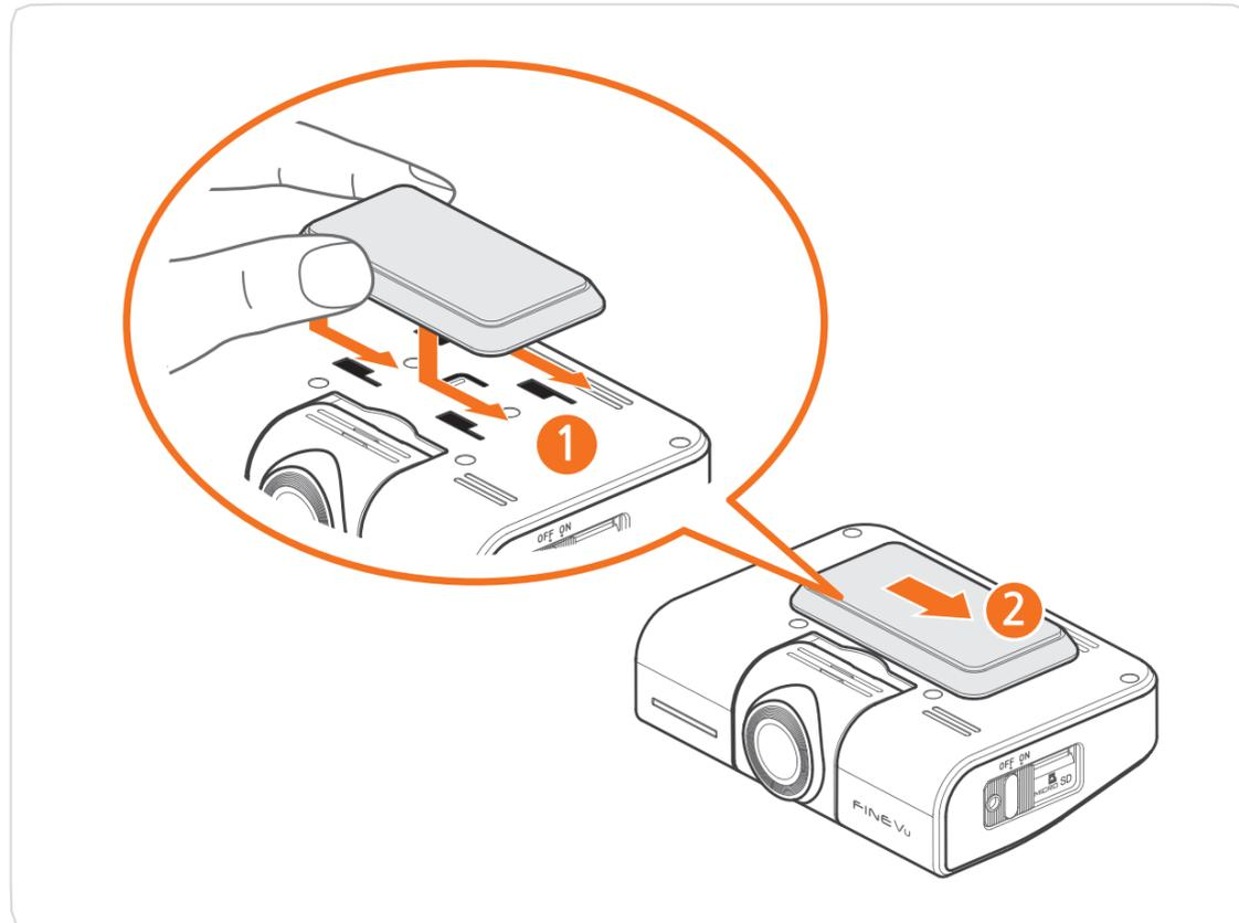
1. Align the cradle part with the arrow ① and insert it into the cradle groove on the main body of the product.
