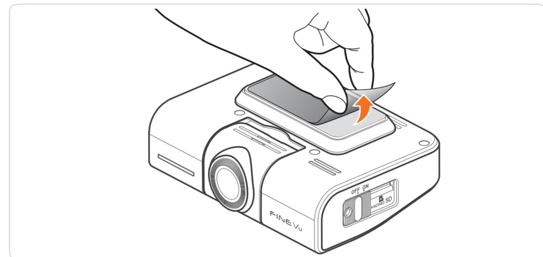
3. Peel off the protective film from the tape for attaching the cradle.
