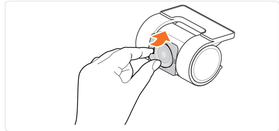
2. Remove the protective film from the rear camera.
