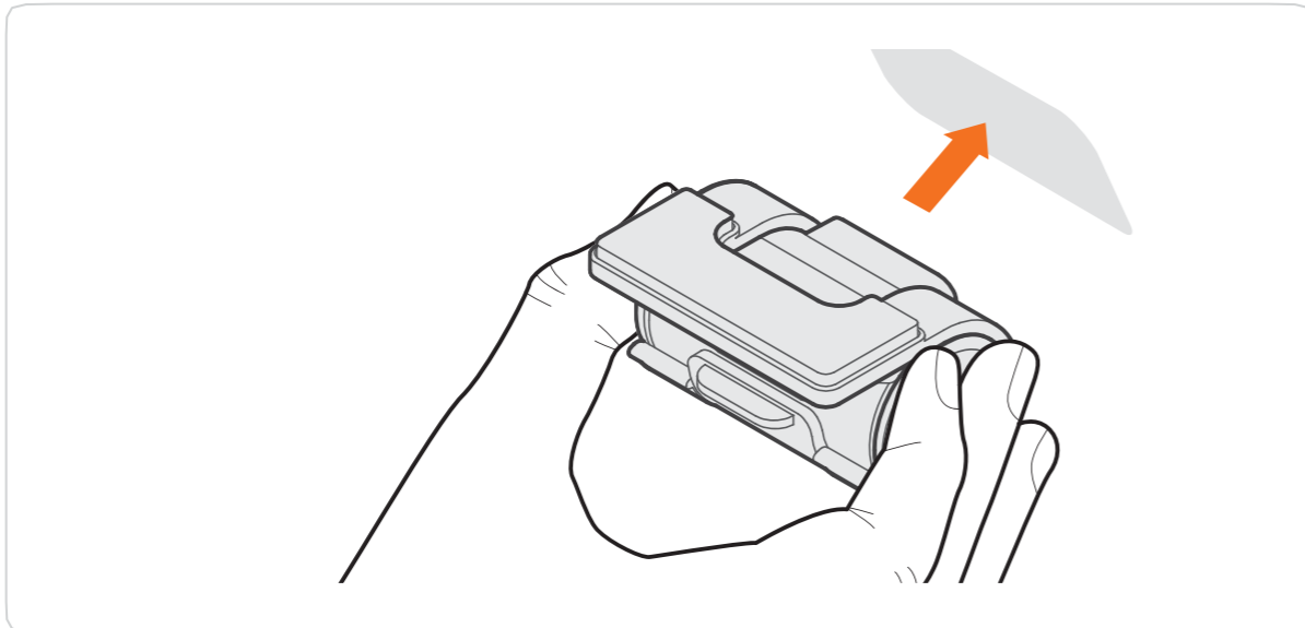
4. Attach the rear camera to the location where you want to install it.
