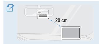
If a GPS navigating device is installed on the dashboard, its GPS reception may be affected depending on the dashboard camera's installation location. Adjust the installation location of the GPS navigating device to ensure that the two devices are separated by at least 20 centimeters (approximately 8 inches).
