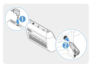
Connect the car charger to the product's DC-IN power port and insert the cigar jack into the vehicle's power socket.
