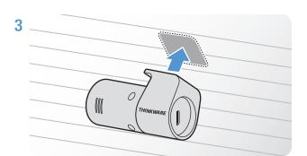
Attach the product with the THINKWARE logo facing indoors and press the adhesive tape firmly to secure the camera.
