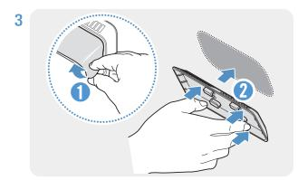
Remove the protective film from the adhesive mount, and then press the mount to the heat blocking film. Push the mount against the windshield to ensure that the mount is firmly fixed.
