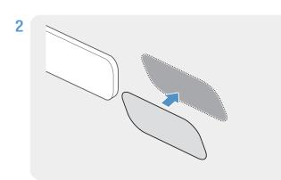
Attach the heat blocking film to the installation location.
