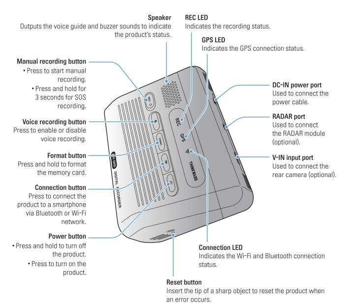
• To reset the product, press and hold the voice recording ( ) and manual recording (REC) buttons simultaneously until you hear beeps.
