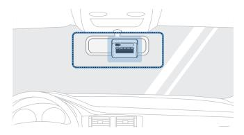
Select an installation location that can record the entire view in front of the vehicle without obstructing the driver's vision. Ensure that the front camera lens is located in the center of the windshield.
