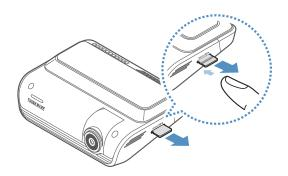
Before removing the memory card, ensure that the product is turned off. Gently push the bottom of the memory card with your fingernail to release it, and then remove it from the product.
